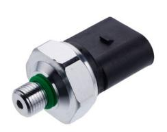
Our oil pressure sensor OPS measures the oil pressure in transmissions of e. g. electric vehicles, in order to optimise the use of the engine power. It was designed to measure the absolute pressure inside the transmission housing, and is robust enough to be used with oil in the surrounding areas.
